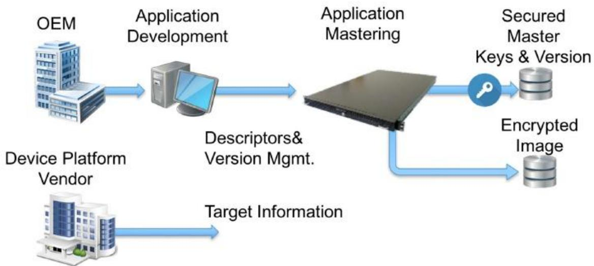
The output of the mastering process is a pair of encrypted files which are loaded into a secure manufacturing process. These secure files can only be decrypted and verified by the Secure Boot Manager that was provisioned with the corresponding master key and product keys.
